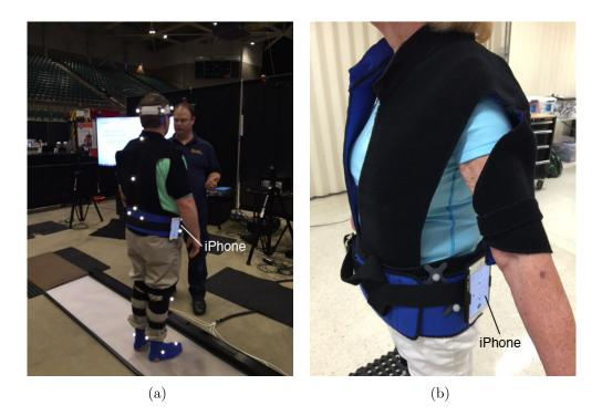
Figure 1: (a) A subject standing on the walkway wearing the custom vest with IR reflectors attached to the back, legs, and feet is also shown fro 3-D motion caption. The right iPhone 6 can be seen attached to the gait belt. (b) Another subject where the left iPhone 6 is shown attached to the gait belt.
