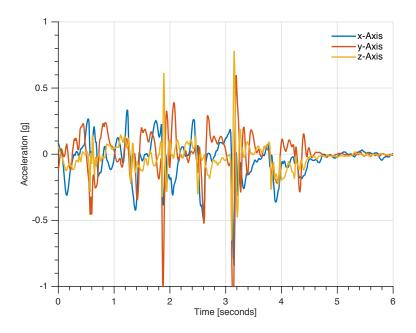
Figure 2: Plot of the raw acceleration signals from the iPhone NM GaitLogger app for all three axes. The periodic nature of the gait signals can be observed in all three axis, where the gait cycle has a period of approximately 1 s.
