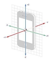
Figure 3: Local coordinate system for iPhone 6 inertial sensors [13]
