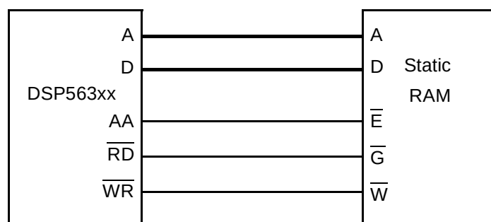
Figure 9-2. Example SRAM Connection Diagram
